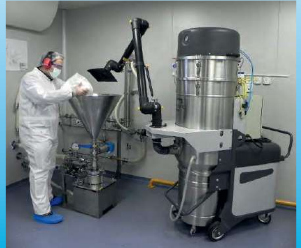
Dosing station dedusting with an ATEX machine fitted with arm and hood
